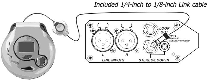
The headphone outputs of portable audio electronics can be connected to the the HX-3 for additional headphone feeds. The included 1/4-inch to 1/8-inch can be used to connect the line-out or headphone output to the HX-3.
