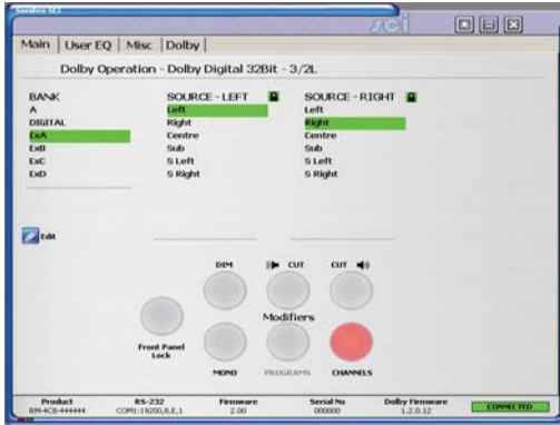
Fig 6-5: Sci Main Screen Showing Dolby Digital Monitoring
