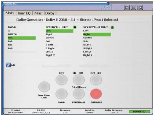
Fig 6-6: Sci Main Screen Showing Dolby E Monitoring
