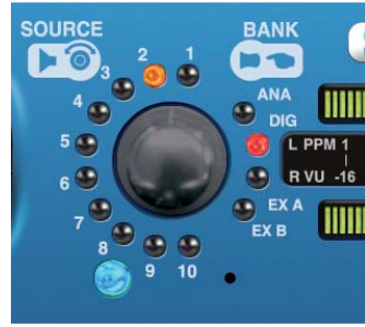
Fig 1-7: RM-2S10 Source Selector
