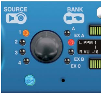
Fig 1-6: RM-2S4 Source Selector
