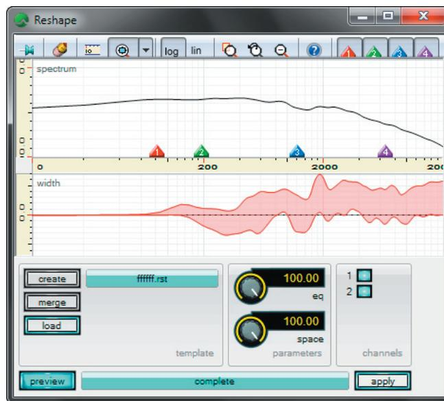
It does so by analysing part or all of a user-defined track to create a template that contains the information about the desired tonal and spatial characteristics. Then, when you define the audio to be processed, it calculates a set of transformation parameters that convert the target's tone and soundstage to that of the template, subject to a pair of controls that allow you to determine the extent of the transformation.
