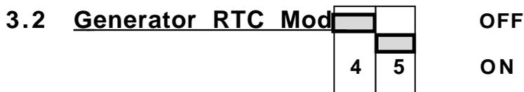
This mode has the same function as the generator-only mode with the difference that on power-up of the master slate the RTC time and date is loaded into the Generator.
