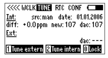
This menu is used to tune (calibrate) other Clockit devices or for the Controller to calibrate its reference oscillator to an external source. The internal reference can be tuned to + - 10ppm with a resolution of 0.15 ppm per digit. The tuning number DAC is shown on the display as well as recent tuning history. The tuning protocol uses an ASCII format connected as cable or through infrared. The tuning process may have
