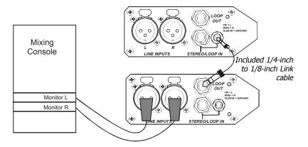
One or more units can be added and "daisy-chained" for additional headphone feeds from a mixing console. Loop additional HX-3 amplifiers with the included Link cable.
