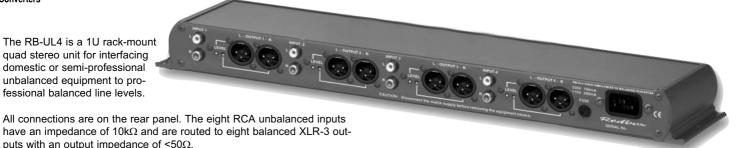
The output gain can be individually adjusted for left and right channels by using pre-set potentiometers accessible through the rear panel.
