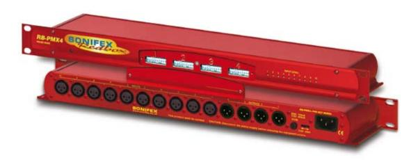
A high performance 10 mono input to 4 mono output pre-set mixer, designed for situations where a small mixer is needed for installations where it will be configured and then only altered occasionally, or never altered at all.
