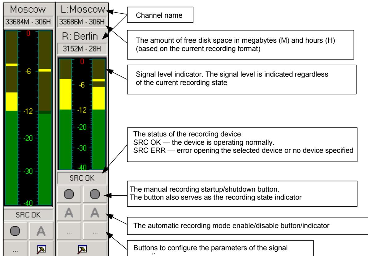
**Fig. 4.** The recording module appearance
