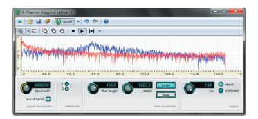
The Single Channel Adaptive Filter removes many forms of interference and background noise, making speech signals more listenable and more intelligible, aiding transcription and making recordings more presentable for the courtroom and juries. Alongside this, the Single Channel Lattice Filter digs deeper into a noisy recording and is capable of extracting more fricative sounds and consonants that would otherwise be buried in noise.
