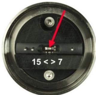
Set the appropriate Bias voltage before mounting the microphone capsule.
