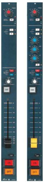
Two balanced stereo inputs with individual gain presets accommodating a wide range of sources including domestic "semi-pro" equipment without additional level matching interfaces. Three-band EQ is optional. Switchable fader start/stop enables smooth sequencing and all remote switching signals are steered through the A/B input selector switch to the active source. Versatile routing can direct the left or right channel to the stereo output or create a mono mix of the stereo input.
